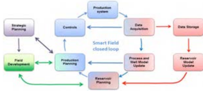
Figure 1: "Closed-loop intelligent field" scheme (Smart Fields Consortium, Stanford University, USA).
