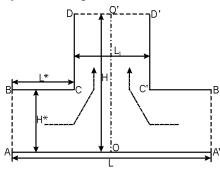
$$\frac{\partial \vec{u}}{\partial t} + (\vec{u}\nabla)\vec{u} + \nabla p = \frac{1}{\text{Re}}\Delta\vec{u} - \frac{Gr\vec{g}}{\text{Re}^2|\vec{g}|}T,$$
