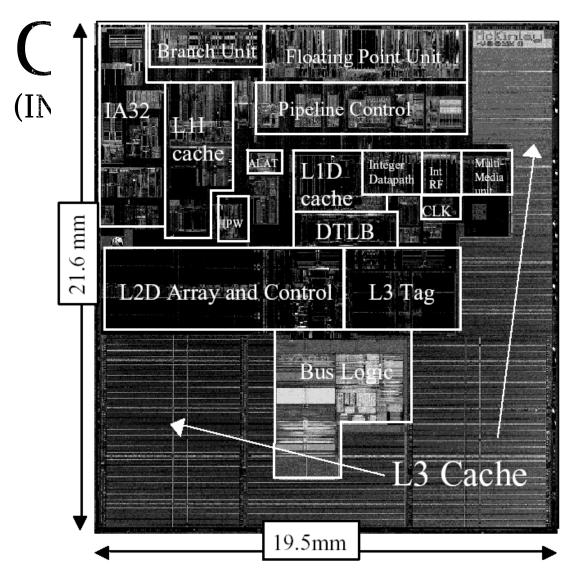
Level 1: 16KB, 4-way s.a., 64B line, quad-port (2 load+2 store), single cycle latency
