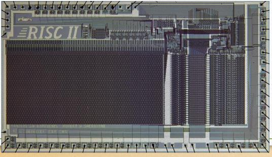
RISC-II (1983) contains 40,760 transistors, was fabbed in 3  $\mu$ m NMOS, ran at 3 MHz, and the size is 60 mm<sup>2</sup>.
