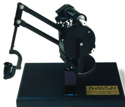
Fig. 1 - A force feedback device called The PHANTOM by SensAble Technologies Inc
