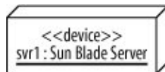
Figure 15-15. Showing the name and type of a node; an instance of a Sun Blade Server named svr1
