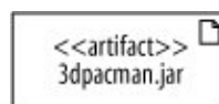
Figure 15-3. A physical software file such as a jar file is modeled with an artifact
