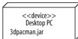
Figure 15-8. A compact way to show deployment is to write the name of the artifact inside the node
