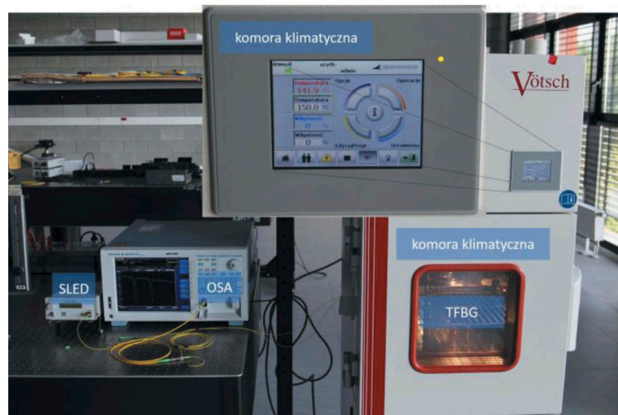
Figure 1. Laboratory stand, used for TFBG temperature measurements.
