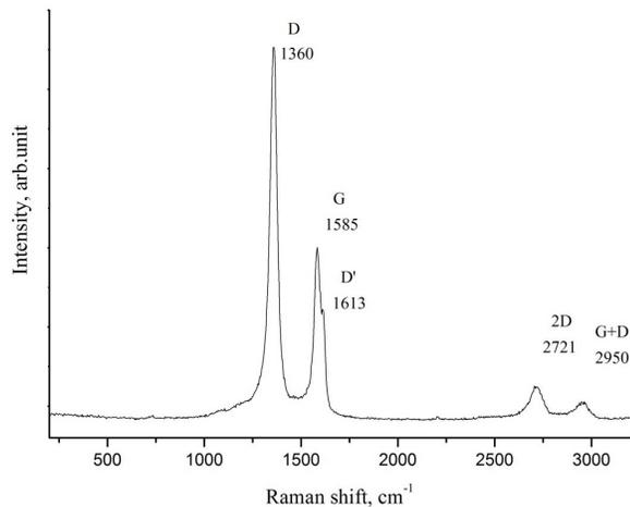
Fig. 1. Raman spectrum of obtained CNWs at RF power of 10 W.
