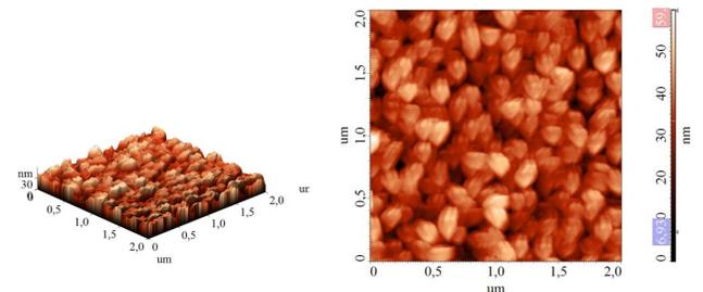
Fig. 5. AFM topography (left) and phase map (right) of synthesized CNWs (sample No. 4) at RF power of 14 W.
