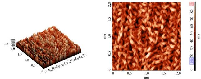
Fig. 3. AFM topography (left) and phase map (right) of synthesized CNWs (sample No. 2) at RF power of 10 W.
