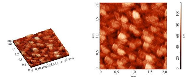
Fig. 4. AFM topography (left) and phase map (right) of synthesized CNWs (sample No. 3) at RF power of 12 W.
