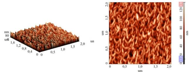
Fig. 2. AFM topography (left) and phase map (right) of synthesized CNWs (sample No. 1) at RF power of 8 W.
