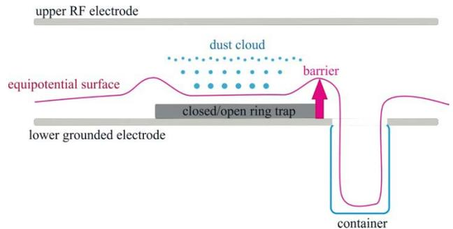
Fig. 4. Formation of a barrier, which prohibits the extraction process.
