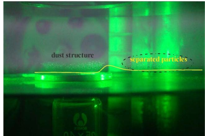
Fig. 6. Extraction of microparticles at the pressure of 0.04 Torr using a closed ring trap. Yellow line: distribution of the lower equipotential surface in RF plasma.
