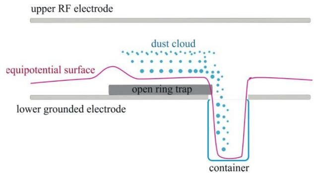
Fig. 3. Distribution of the equipotential surface in the RF plasma near the bottom electrode.
