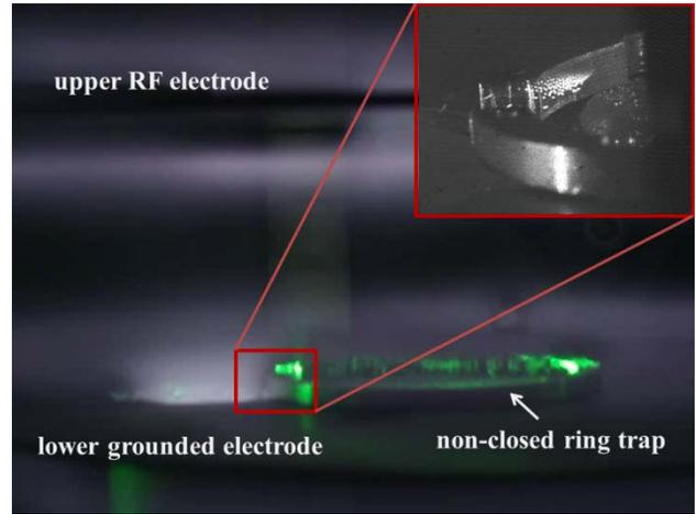
Fig. 2. Extraction process of levitated microparticles from the dust cloud. Red square: flow of microparticles falling down into the container.
