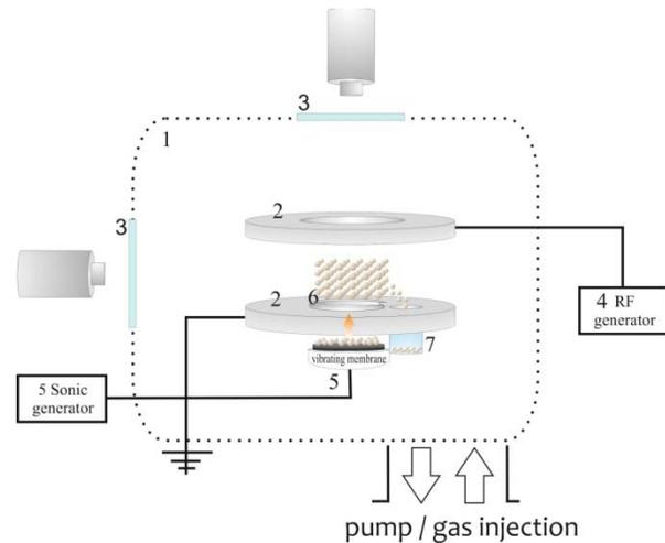
Fig. 1. Scheme of the experimental setup for investigation of the dust structure behavior.
