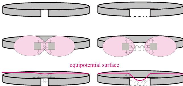
Fig. 5. Difference between the electric fields of two different open ring traps at the same value of RF power. Arrows: plasma sheath length (characteristic screening length of the ring field).
