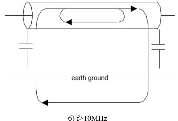
**Figure 6 – Shielding current paths depending on the frequency of the interference**
