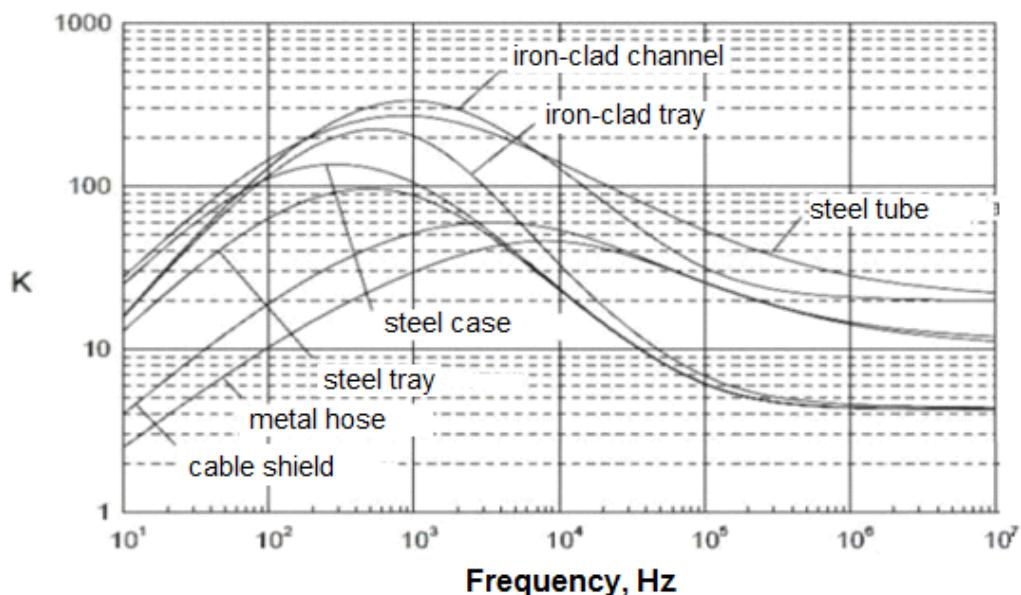
**Figure 4 – Dependence of the shielding coefficient of various elements on the frequency of the SMI**
