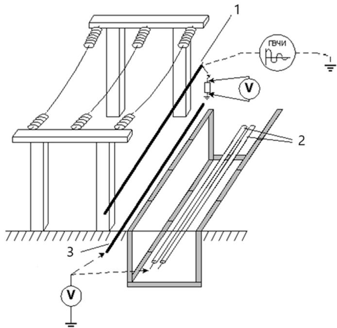
**Figure 7** – Scheme for simulating radiated impulse noise.
