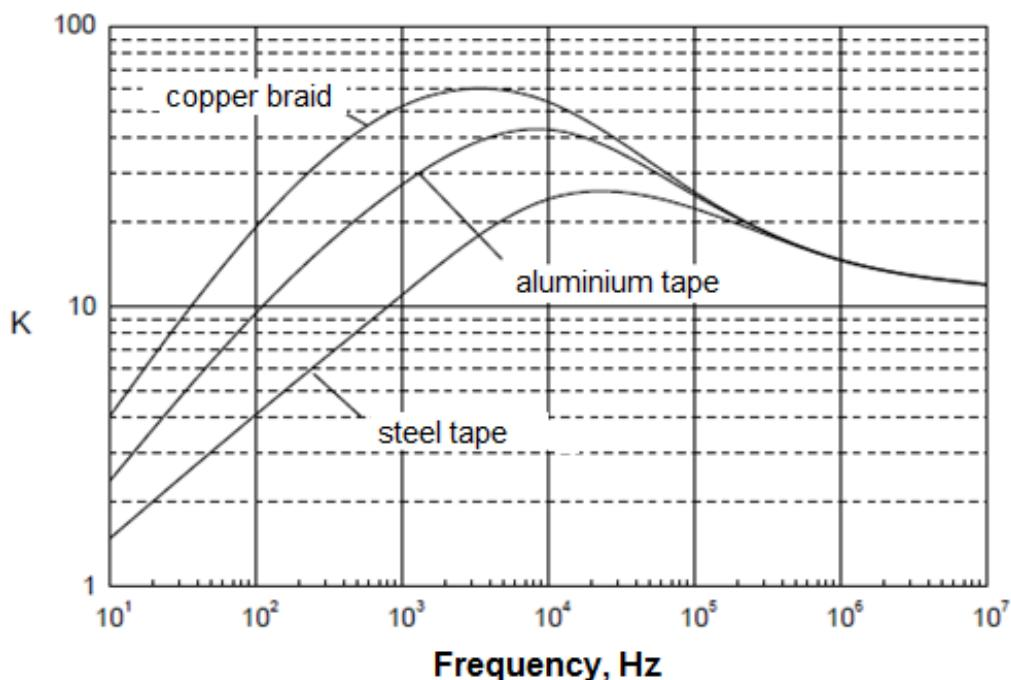
Figure 5 – Shielding factors for cable screens
