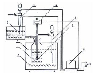
Fig. 1. A scheme of the laboratory installation: 1 - a reactor; 2 - a thermostat; 3 - a contact thermometer; 4 - a temperature relay; 5 - a mixer; 6 - an electric motor; 7 - a hotplate.
