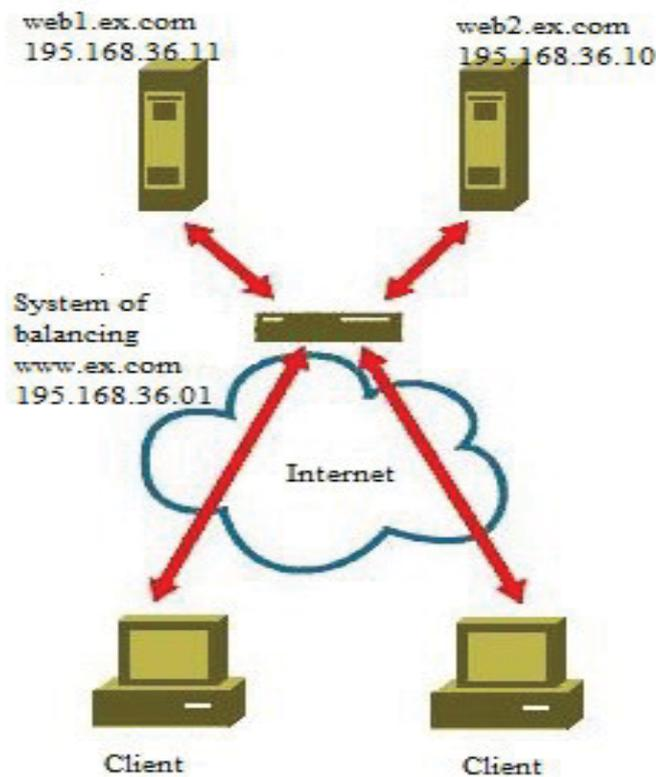
Figure 1. Balancing system
